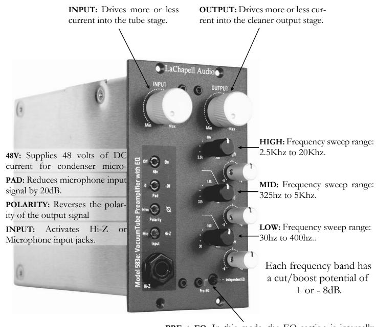
**PRE + EQ:** In this mode, the EQ section is internally routed to serve the preamp's output signal; effected signal is sent out the left bay output jack.
